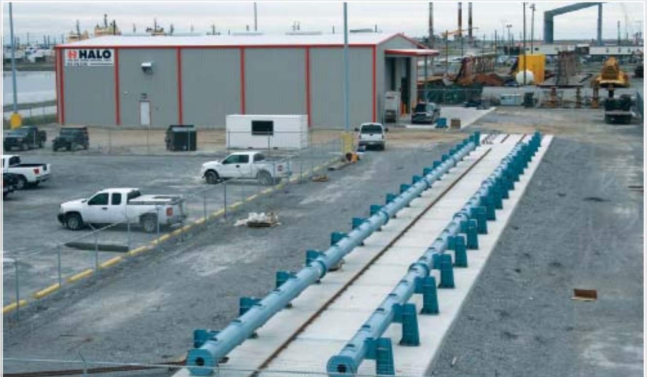
The Halo LLC facility in Port Fourchon is equipped with a 3-million lb (1,361-metric ton), 220-ft (67-m) load test bed to test all sizes and types of mooring lines and heavy-lift slings.
